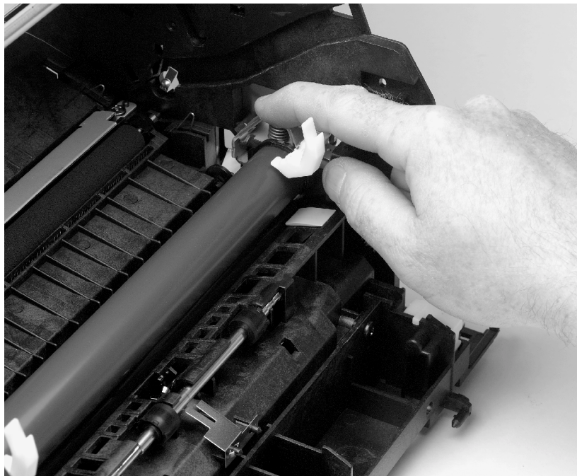
Figure 47. Fusing element metal clips reinstallation
